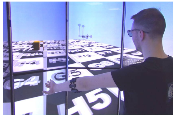
Figure 3. Integration of MYO armband to operate with 3D object.
